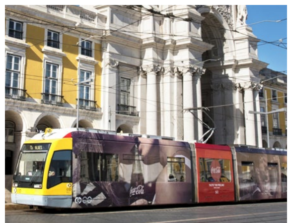
Sécheron's SPL pantograph integrated on an existing tram.
