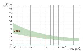
Relationship between opening time  $t_1$  and the initial rate of rise of current di/dt for direct instantaneous over-current release.
