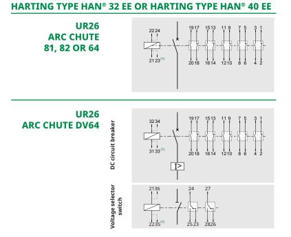
Circuit breaker main contact Voltage selector switch main contact Closing coil  $\square$ Low voltage connector interface \_\_\_\_ (male pin) |> Overcurrent tripping a 🖓 b 1a+1b - Switch CO a b 1a+1b - Switch PF only for 24 V
