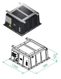
The insulation housings have to be ordered additionally to the DC circuit breaker (see page 12).
