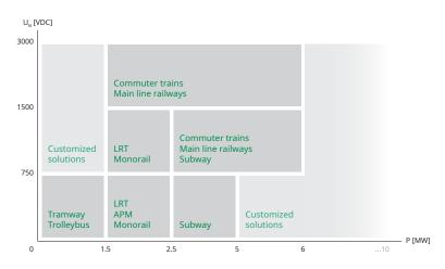
Thanks to its complete range of rated voltages, Sécheron is able to cover all types of traction networks. With many years of experience in the field, Sécheron is able to propose a reliable and suitable range of diode rectifiers for DC traction power supply. Our natural air cooled rectifiers are equipped with diode blocks with high overload capability and high blocking voltage.
