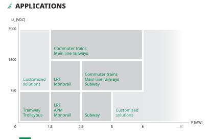
Thanks to its complete range of rated voltages, Sécheron is able to cover all types of traction networks. With many years of experience in the field, Sécheron is able to propose a reliable and suitable range of diode rectifiers for DC traction power supply. Our natural air cooled rectifiers are equipped with diode blocks with high overload capability and high blocking voltage.
