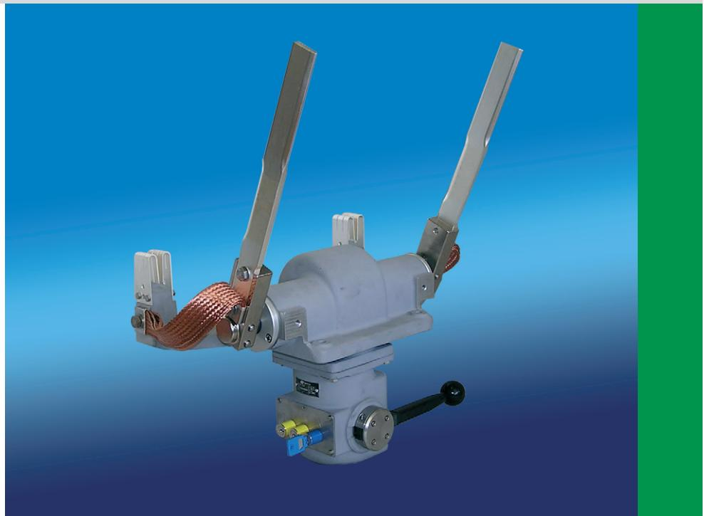
The **BTE** earthing switch is a double pole, manual operated device with safety interlocking keys, designed to ground the circuits on both sides of the roof mounted AC vacuum circuit breaker type BVAC.
